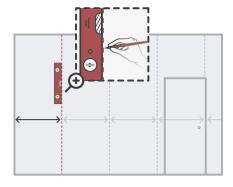
Put a mark close to the ceiling at this point. This is where you start your spirit-level or plumb-line from and will allow half an inch overlap around the corner. Mark down the plumb-line every 11-15". This will give you a good vertical line to hang your first length to, USE PENCIL ONLY.
