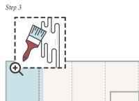
Our wallpapers are made using a non-woven base, that means you apply the adhesive directly to the wall. Start by pasting an area sufficient enough to cover just over one drop width at a time.
