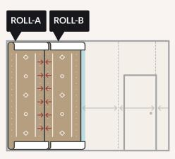
Butt join the **Roll A** length and the **Roll B** length together, matching up the edges.
