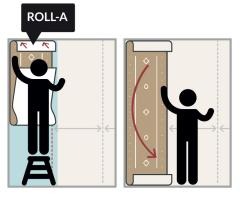
Attach the top of the length to the wall at the preferred height and in the correct position before letting go of the rest. Align the top and bottom of the first length before "smoothing down" the wallpaper.
