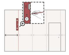
Put a mark close to the ceiling at this point. This is where you start your spirit-level or plumb-line from and will allow half an inch overlap around the corner. Mark down the plumb-line every 11-15". This will give you a good vertical line to hang your first length to. USE PENCIL ONLY.
