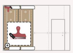
When you're happy with the position, using a straight edge, trim the excess wallpaper at the top and bottom of the wall. Use a sharp snap off blade knife. Push the paper into the ceiling line and skirting.
