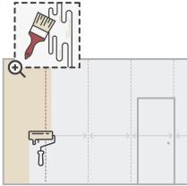
Our wallpapers are made using a non-woven base, that means you apply the adhesive directly to the wall. Start by pasting an area sufficient enough to cover just over one drop width at a time.
