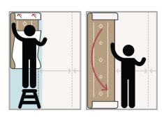
Attach the top of the length to the wall at the preferred height and in the correct position before letting go of the rest. Align the top and bottom of the first length before "smoothing down" the wallpaper.
