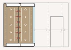
Butt join the lengths of wallpaper together, matching up the edges. Ensure that the lengths are properly positioned, that the pattern is matching and there is no surface visible at the joints.
